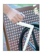
**6.** Raise the ramp by turning the gearbox crank clockwise until the ramp is firmly against the back of the rear wheels of the wheelchair.
