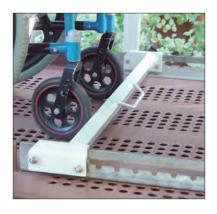
**7.** Adjust the front Stop Bar to secure against the front wheels of the wheelchair. NOTE: It may be necessary to remove the wheelchair foot-rests or tilt the chair to raise the foot-rests over the Stop Bar so the front wheels are secured against the Stop Bar.
