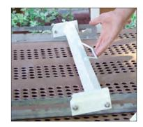
**2.** Adjust the Stop Bar to allow adequate space for the wheelchair.
